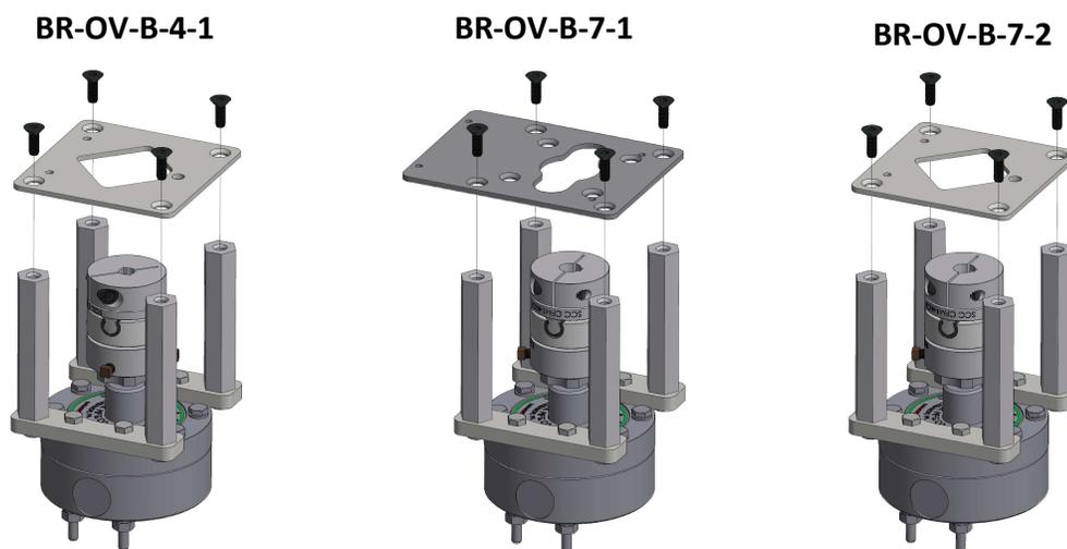
**Figure 7: Actuator Mounting Bracket Installation**
