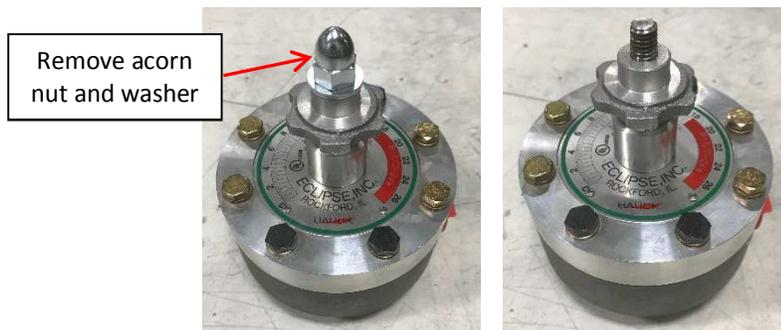
**Figure 2: Acorn Nut and Washer Removal**
