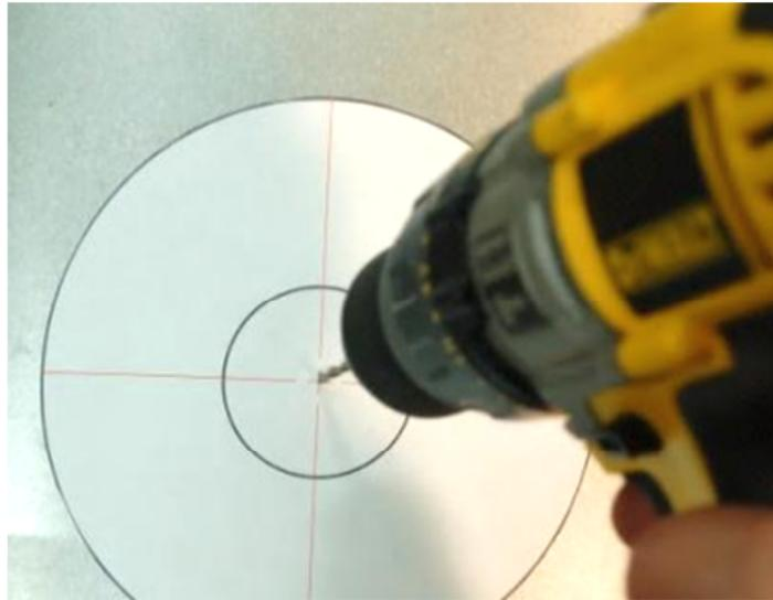
**Figure 3: Sticker Placement and Pilot Hole Preparation**
